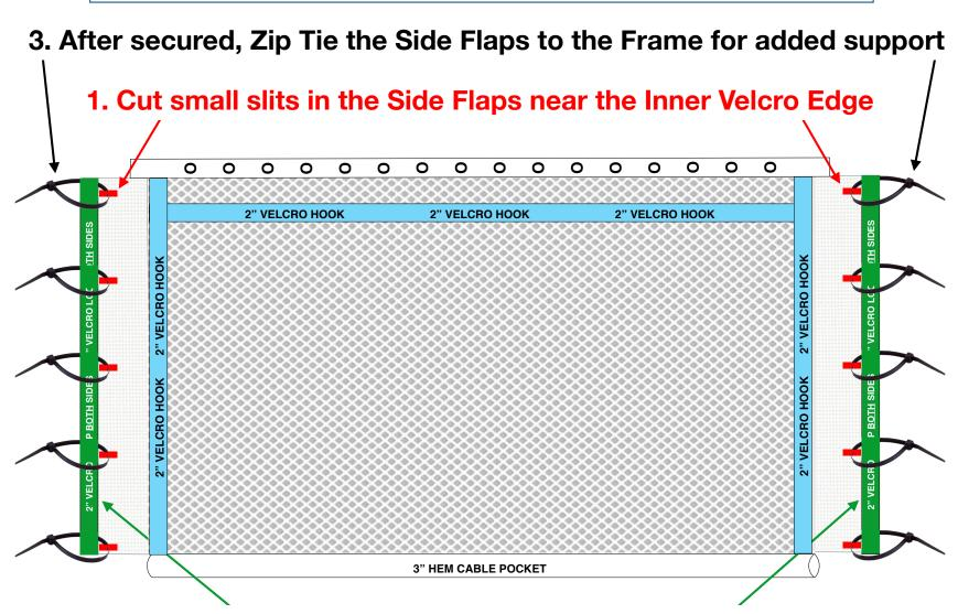
2. Secure the Velcro Loop to the Velcro Hook on the Vertical Beams of the Frame
